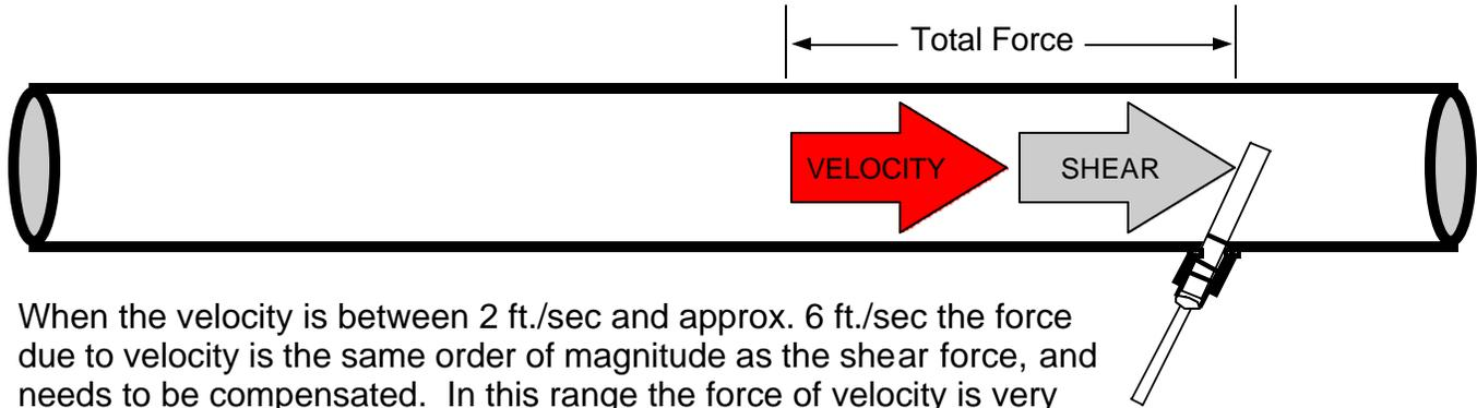
When the velocity is between 2 ft./sec and approx. 6 ft./sec the force due to velocity is the same order of magnitude as the shear force, and needs to be compensated. In this range the force of velocity is very predictable and reproducible, and can be compensated accordingly, removing it from the shear force measurement.
