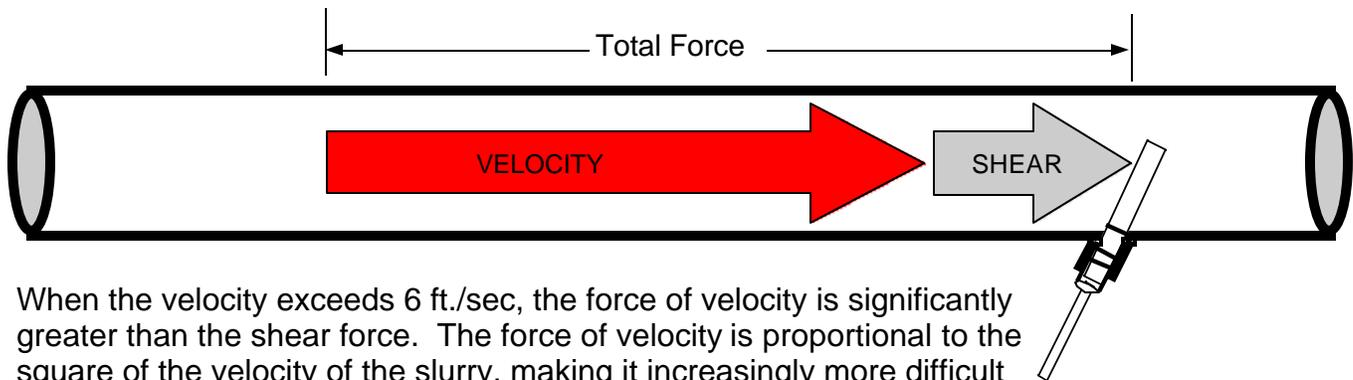
When the velocity exceeds 6 ft./sec, the force of velocity is significantly greater than the shear force. The force of velocity is proportional to the square of the velocity of the slurry, making it increasingly more difficult to compensate, overwhelming the shear force measurement.
