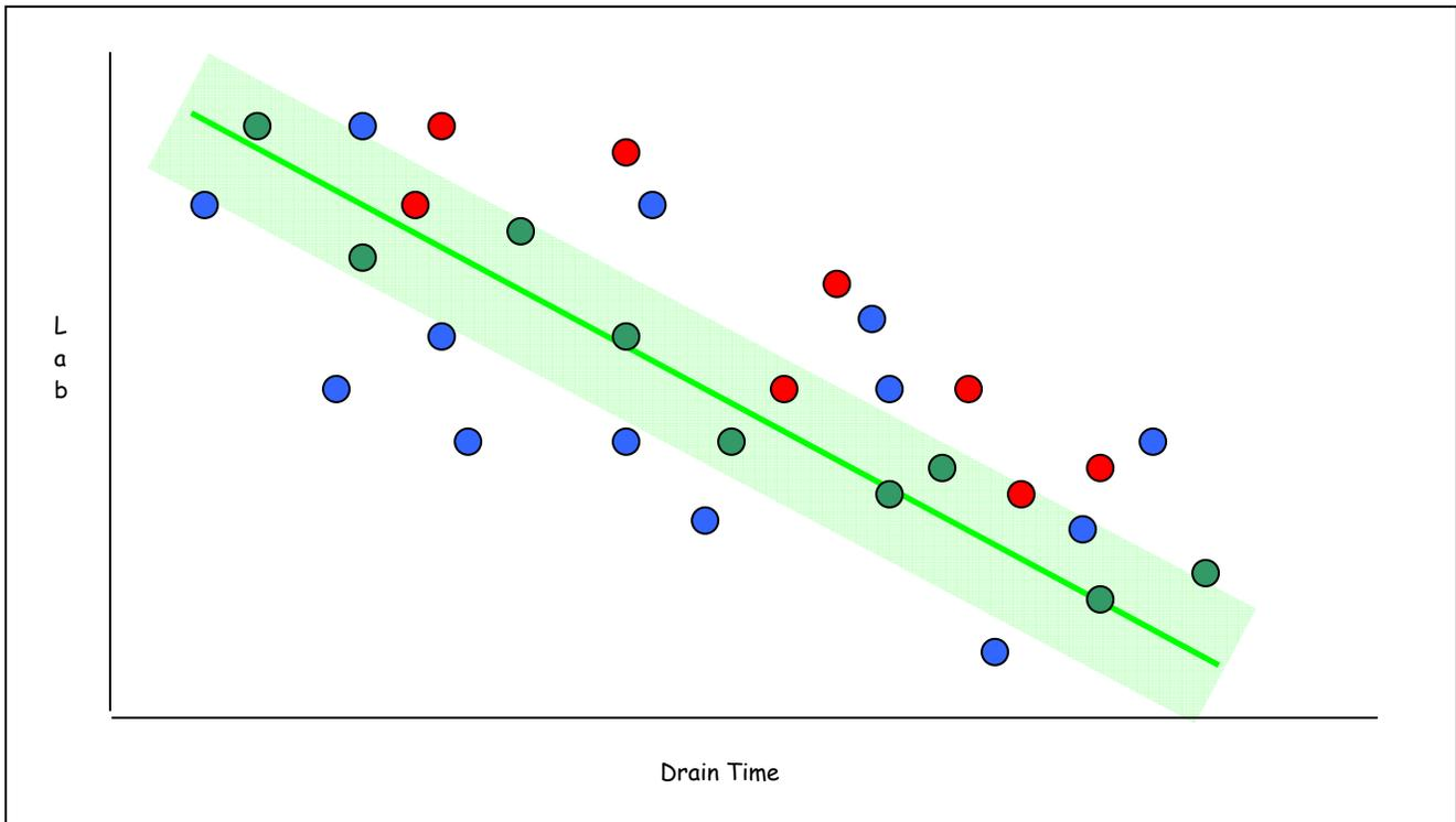
In the figure above, the green line represents the best fit calibration line developed by regression of laboratory and Drainac data. The shaded green area represents the  $2\sigma$  limits of acceptable variation as defined by the statistics of the regression.
