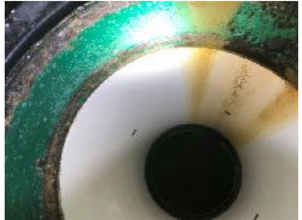
This TECO SAM had 500,000,000 pounds of sand flow through its core. Upon inspection, the customer found the flow tube to be looking "brand new".
